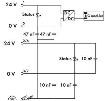
This internal system supply module increases the current supply for the internal system by 2 A.
