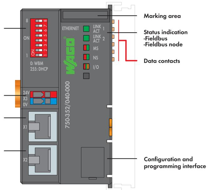
The 750-352 ETHERNET Fieldbus Coupler connects ETHERNET to the modular WAGO-I/O-SYSTEM.
