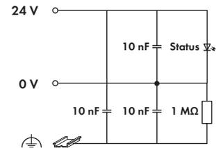
This supply module provides the I/O modules with the corresponding supply potential. Maximum available supply current to all connected modules is 10 A. When configuring the system, it must be ensured that this total current is not exceeded. Should higher currents be necessary, an intermediate supply module must be added to the assembly.
