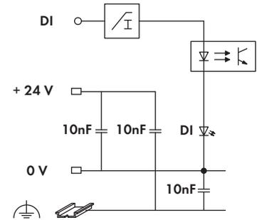
This 2-wire digital input module provides 8 channels at a width of just 12 mm. It receives binary control signals from digital field devices (e.g., sensors, encoders, switches or proximity switches). The module features CAGE CLAMP® S connections providing push-in termination of solid conductors. Each input channel has a noise-rejection RC filter with 3.0 ms time constant. A green LED indicates the switched status of each channel. Field and system levels are electrically isolated.
