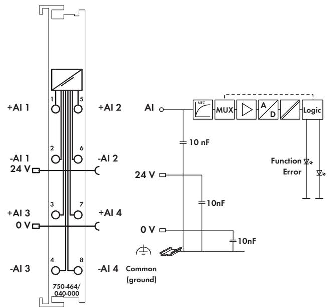
The input module directly connects to Pt or Ni resistance sensors and potentiometers. It can be operated as a 2-channel (2- and 3-wire technology) or 4-channel (2-wire technology) module. The bus module linearizes the entire temperature range. A sensor error (short circuit, line break or measuring range overflow) is indicated by a red LED. The module can be configured via WAGO-I/O-CHECK or GSD files. The module features multiple setting options and high accuracy.
