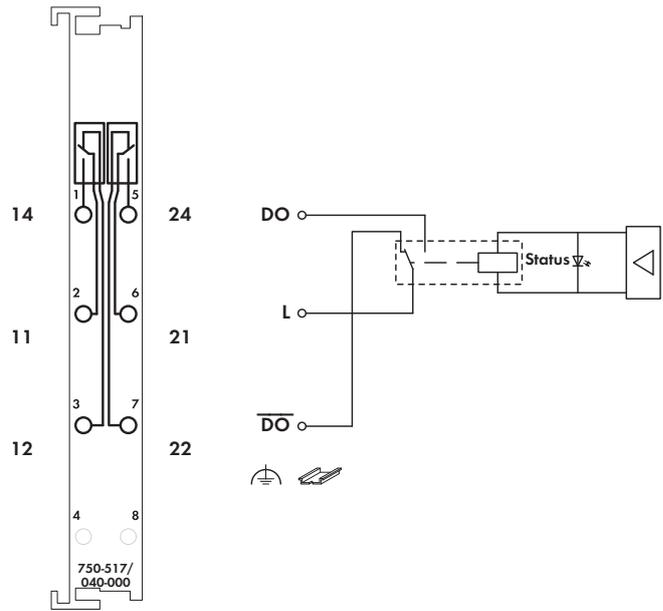
This digital output module transmits control signals from the automation device to the connected actuators.
