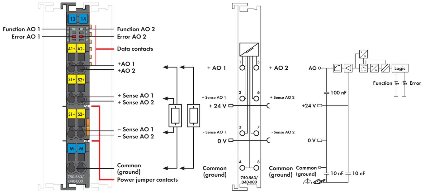
This analog output module generates 0/4–20 mA output currents or 6–18 V output voltages for the field.
