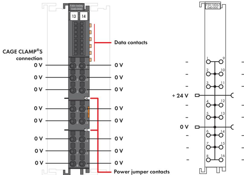
This field-side connection module is used in combination with the 16-channel 750-1504 Output Module (also suitable for 8-channel output modules with a single conductor connection) for providing the 0 V potential to the outputs. This eliminates the need for additional terminal blocks.
