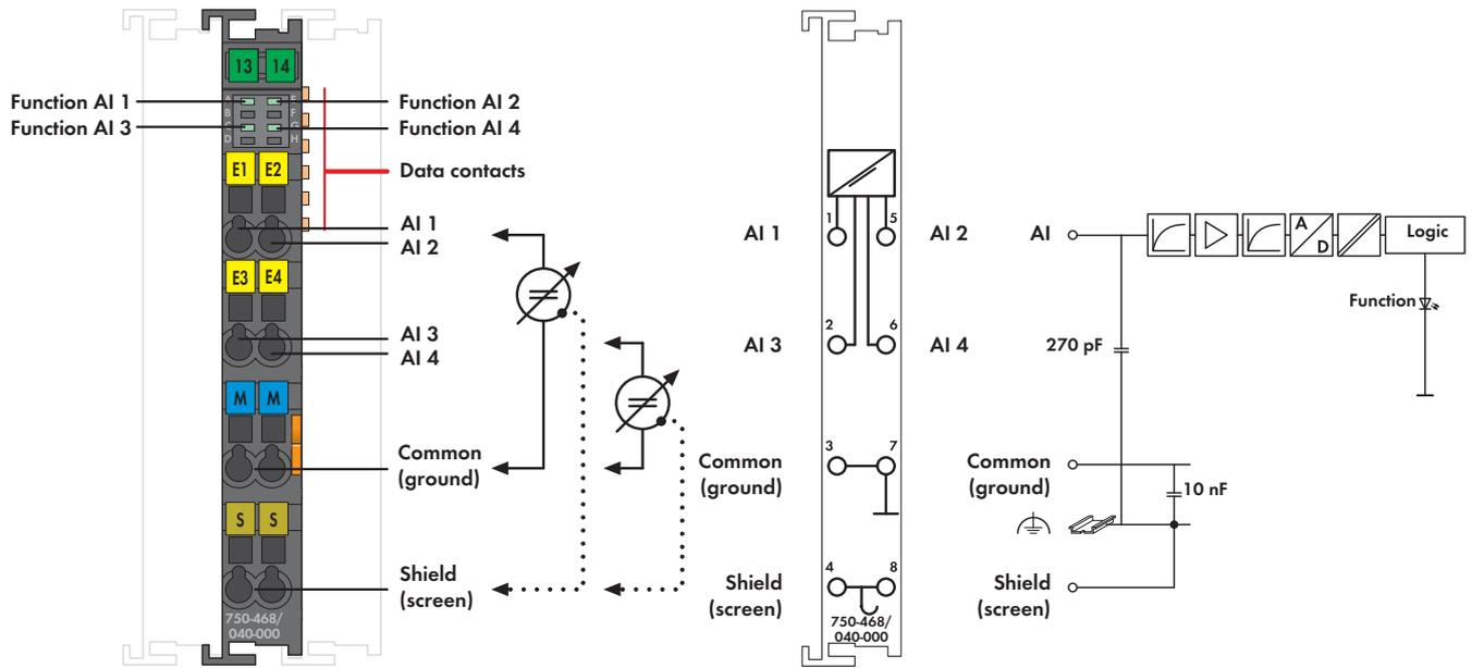
The analog input module processes standard 0-10 V signals. The input signal is electrically isolated and transmitted with a resolution of 12 bits.
