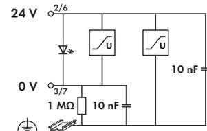
The WAGO-I/O-SYSTEM 750 can also be used in shipbuilding applications and onshore/offshore installations (e.g., platforms, loading facilities). This is possible via certification under the standards of leading agencies such as Germanischer Lloyd and Lloyds Register. Proper system operation is ensured (certified) by using this overvoltage protection module. This module is equipped with surge suppression and can also be used as a power supply module.
