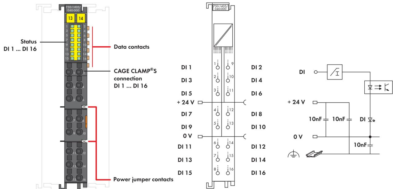
This digital input module provides 16 channels at a width of just 12 mm. It receives binary control signals from digital field devices (e.g., sensors, encoders, switches or proximity switches). The module features CAGE CLAMP® S connections providing push-in termination of solid conductors. Each input channel has a noise-rejection RC filter with 3.0 ms time constant. A green LED indicates the switched status of each channel. Field and system levels are electrically isolated.
