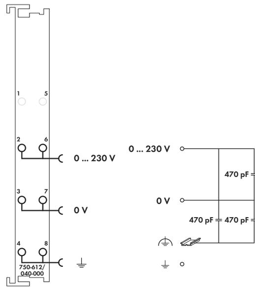
This supply module provides the I/O modules with the corresponding supply potential.
