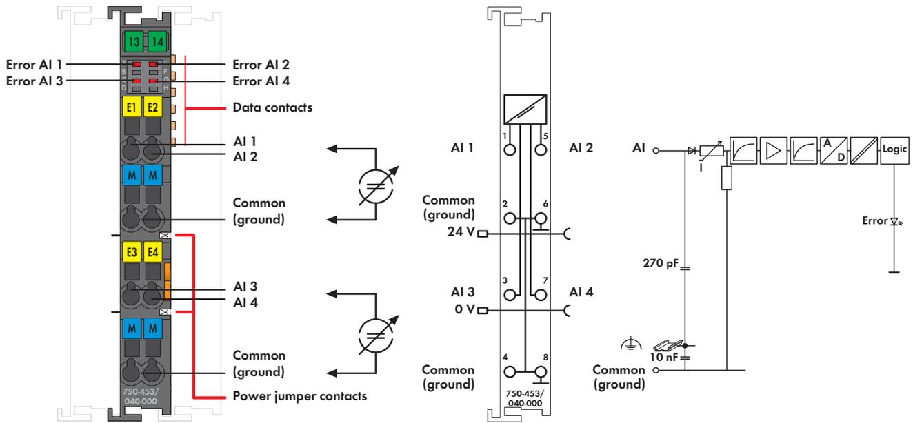
The analog input module processes standard 4–20 mA signals. The input signal is electrically isolated and transmitted with a resolution of 12 bits. The internal system supply powers the module. The input channels of the module have a common ground potential.
