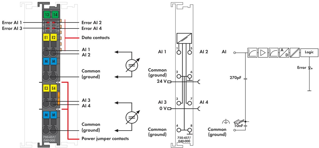
This analog input module processes standard ±10 V signals. The input signal is electrically isolated and transmitted with a resolution of 12 bits. The internal system supply powers the module. The input channels of the module have a common ground potential.
