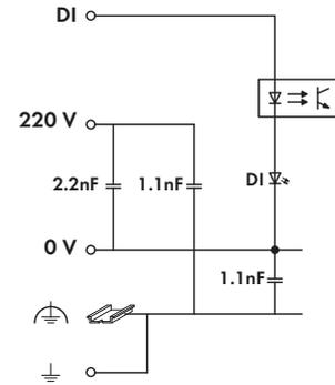
The digital input module receives control signals from digital field devices (e.g., sensors). The module is a 4-conductor device allowing direct connection of sensors with ground contact. Each input module has a 3.0 ms noise-rejection filter. Field and system levels are electrically isolated. The field power must be reapplied after every 7 modules.
