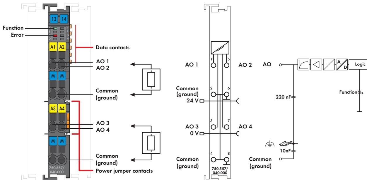
This analog output module generates standard  $\pm 10\text{ V}$  or  $0\text{-}10\text{ V}$  signals. The output signal is electrically isolated and transmitted with a resolution of 12 bits. The internal system supply powers the module. The output channels of the module have a common ground potential.
