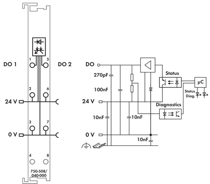
This digital output module transmits control signals from the automation device to the connected actuators. All outputs are short-circuit proof. This output module detects the following errors: overload, short-circuit and wire break. The status is transmitted to the fieldbus coupler and indicated by LEDs. The module is a 4-conductor device and actuators with ground connection may be directly connected to it.
