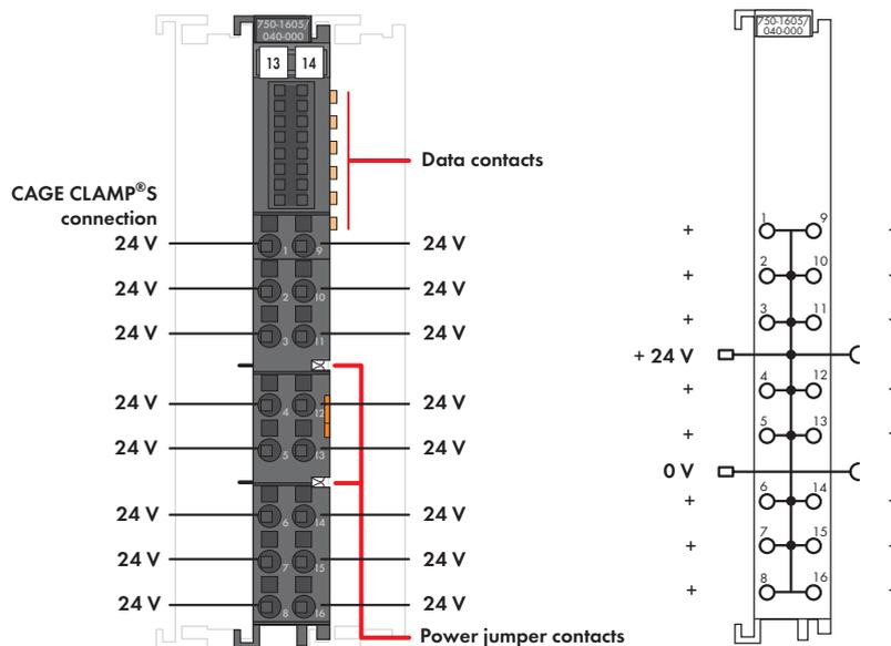
This field-side connection module is used in combination with the 16-channel 750-1405 and 750-1406 Input Modules (also suitable for 8-channel input modules with a single conductor connection) for providing the 24 V potential to the inputs.
