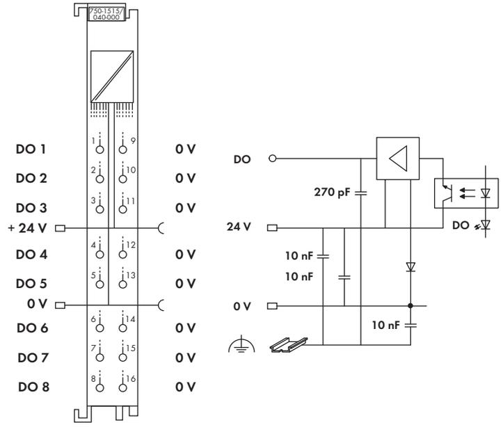
This 2-wire digital output module provides 8 channels at a width of just 12 mm. It transmits binary control signals from the automation device to the connected actuators (e.g., magnetic valves, contactors, transmitters, relays or other electrical loads). The module features CAGE CLAMP® S connections providing push-in termination of solid conductors. A green LED indicates the switched status of each channel. Field and system levels are electrically isolated.
