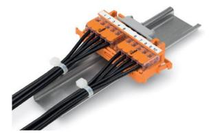
Four different mounting options are possible with the new mounting carrier. The simplest method is snapping the carrier vertically onto the DIN-rail, or, as shown here, mounting it horizontally on the DIN-rail using a 222 Series Angled DIN-Rail Adapter (222-510). The carrier can also be screwed to smooth, flat surfaces if necessary.
