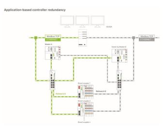
WAGO concept for applicative controller redundancy
