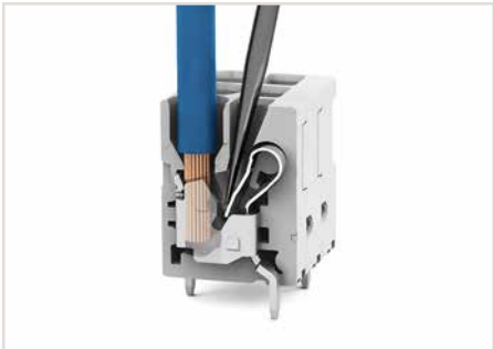
Insert solid conductors via push-in termination. Insert fine-stranded conductors – as well as remove all conductors – via operating tool.
