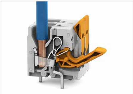
Insert solid conductors via push-in termination. Insert fine-stranded conductors – as well as remove all conductors – via operating lever.
