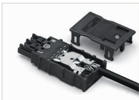
First insert wired connector into strain relief housing, then snap cover and tighten screw.
