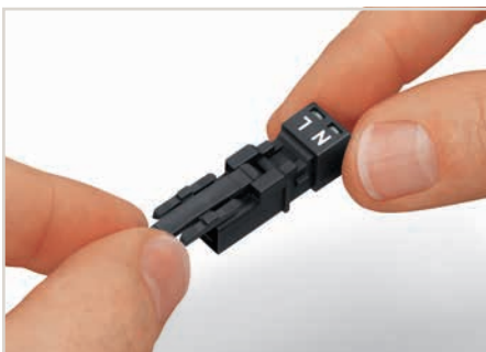
All connectors for fixed installations (snap-in versions, pluggable PCB connectors, distribution connectors) are factory-equipped with locking levers to ensure plugs and sockets are securely locked. Additional locking levers are only required for "flying leads" (plug/socket).
