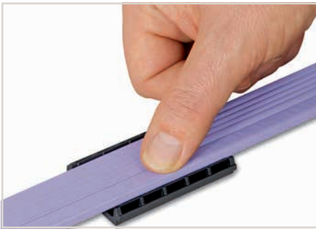
Insert flat cable into base (observe coding!).
