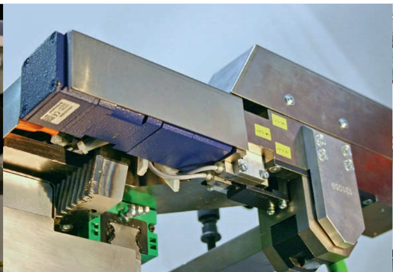
2. The positioning via stepper motors must allow printing with precision.
