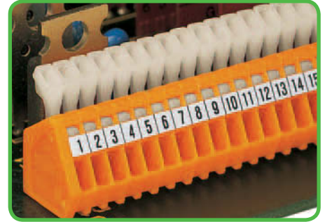
Marking via self-adhesive strips or factory direct printing.
