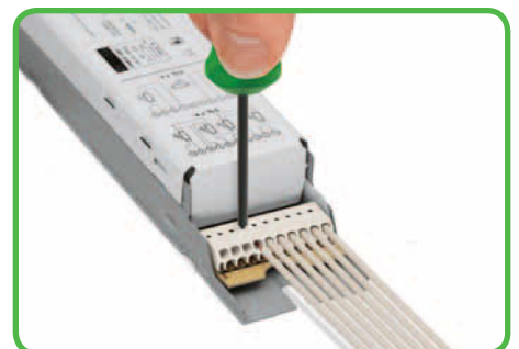
Removing conductor via Ø 1.0 mm disconnection tool.
