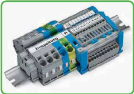
Each connection point features an individual marker slot for WMB markers. Additionally, the upper marker slot is suitable for marker strips that can be marked manually using a felt-tip pen or automatically via thermal transfer printer.
